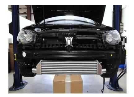
Since there are no pre-existing mounting holes on the MK6 application, the hole locations will need to be marked and drilled. <u>Please reference the pictures below.</u>
