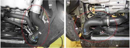
Remove the doubled o-ring seals from the original intercooler hoses and fit these to the included corresponding new aluminium hose couplings as pictured below.
