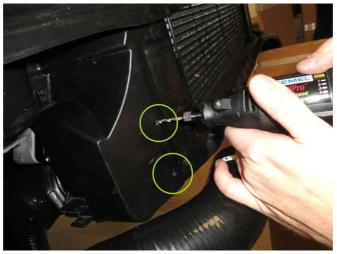
With the mounting holes drilled, position the Forge intercooler core in place and secure it using the supplied self-tapping screws and washers. If you encounter any resistance tightening the screws, please check the available depth of the hole to ensure that you are
